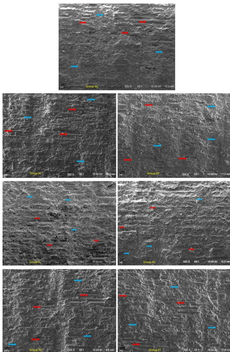
**Figure 1.** SEM photographs of post surfaces in different experimental groups at 500X magnification show areas of epoxy resin (→) and some areas of exposed fibers (→).
