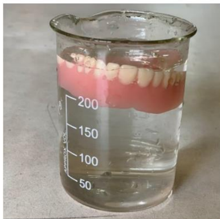
Figure 5: Light weight hollow denture.
