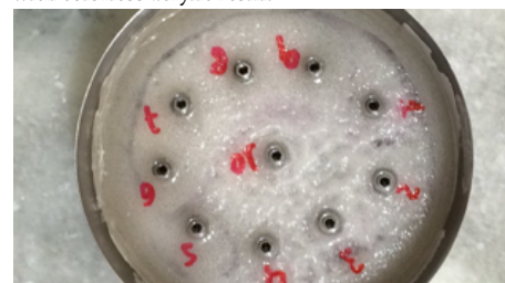
Figure 1. Specimens set on the metal bowl filled with colorless acrylic resin.
