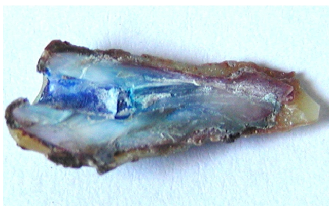
Figure 6. Photograph showing dye penetration in experimental group with hybrid composite as cervical base.
