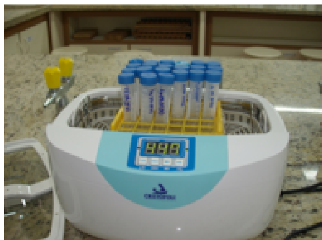
Figure 4. Ultrasound tank. Tubes with specimens are sonicated in order to provoke disintegration of bacterial biofilm.
