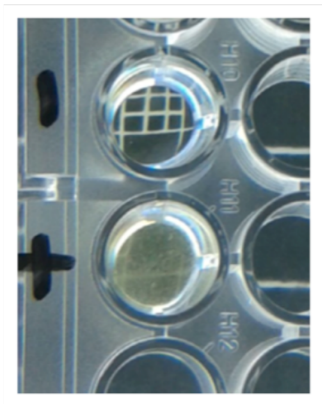
Figure 4. Titer plate showing the positive control solution (+) TSB + bacteria and the negative control (-) TSB pure.
