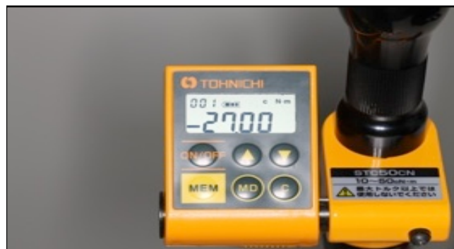
Figure 3: Measure of reverse torque values of abutments by digital wrench.
